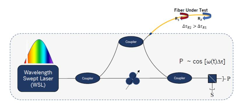
Where:  $\Delta \tau$  path delay difference  $\omega$  optical frequency
