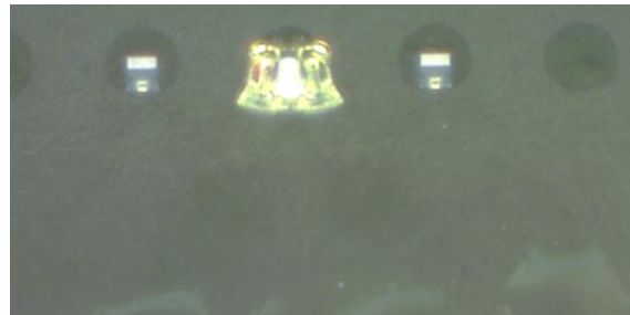
3D-printing of 3 periscope lenses on MCF terminated in a MT ferrule
